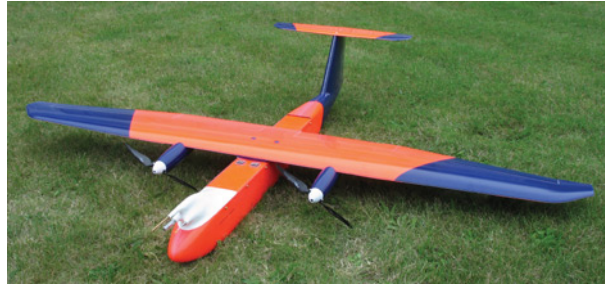
Fig. 1 CAROLO T200: a fully automatic small UAV, 2 m wingspan, 5 kg maximum takeoff weight, 2 kg payload (pictured here with wind measuring 9-hole-probe and other meteorological sensors).
